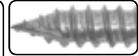
The Type 17 point will clean the existing hole of metal burrs & the oversized threads will generate increased holding strength.
